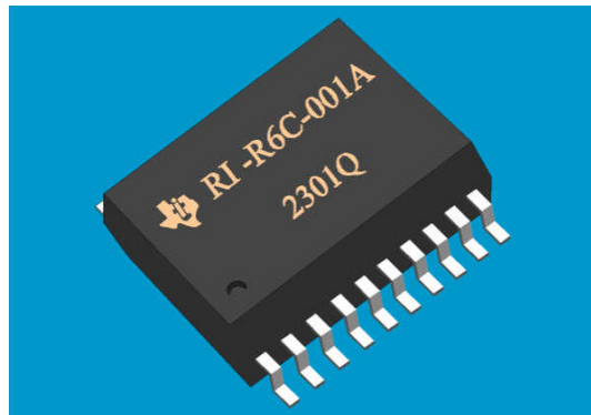
Figure 1: S6700 Multi Protocol Transceiver IC (RI-R6C-001A)
